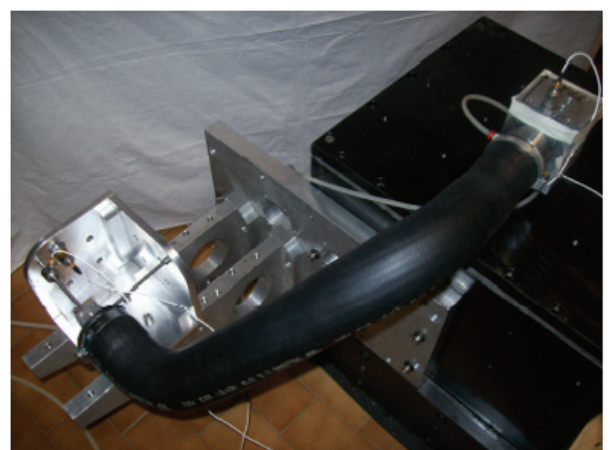
Fig. 3: Hydraulic shaker measuring the dynamic matrix of a flexible hose
