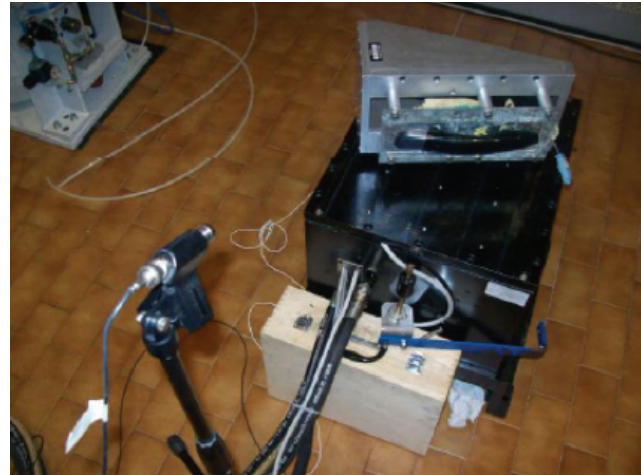
Fig. 1: Hydraulic shaker during a S&R test
