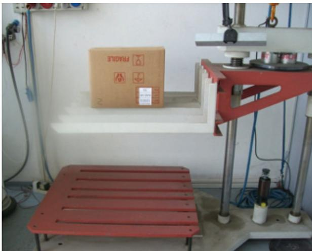
Fig. 1: Drop Test Machine during packaging testing
