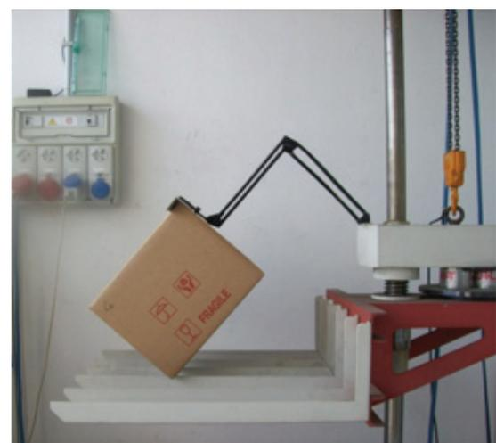
Fig. 3: Drop Test Machine during packaging testing
