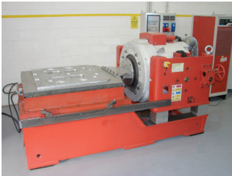
Fig. 1: V895 shaker with slip table - configuration for testing on horizontal axis
