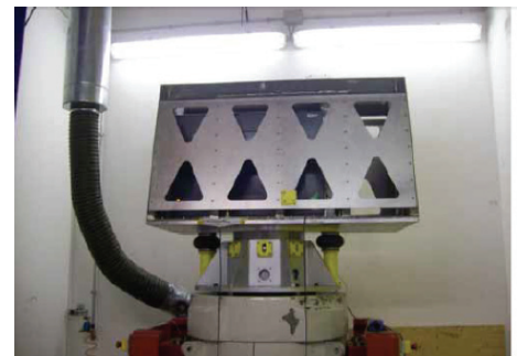
Fig. 2: Detail of fixture mounted on the shaker
