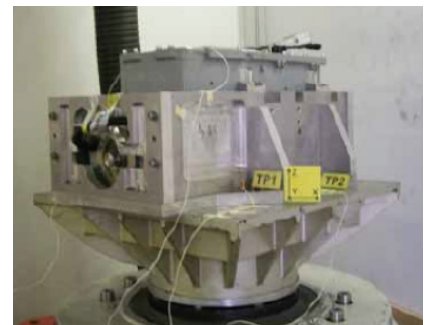
Fig. 3: Detail of fixture mounted on the shaker
