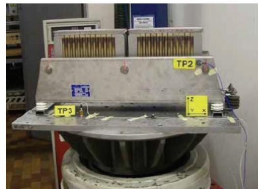
Fig. 2: V850 shaker during a railway vibration testing (vertical axis)
