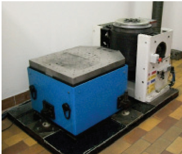
Fig. 1: V724 shaker with slip table
