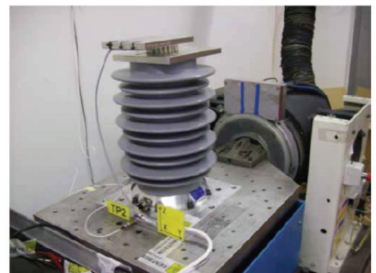
Fig. 3: V724 shaker during tests with slip table
