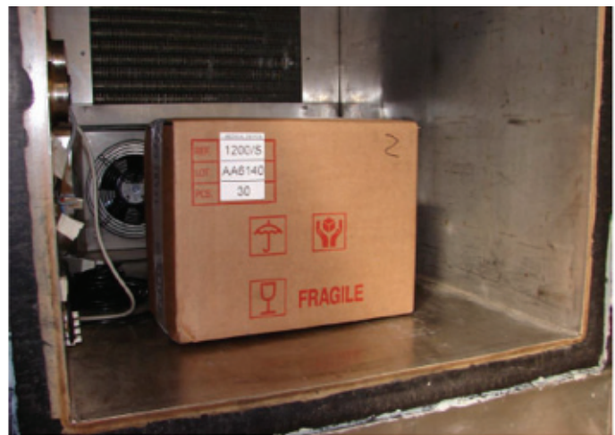
Fig. 1: Altitude chamber, view from inside with the item to test
