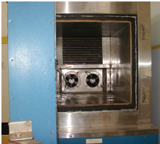
Fig. 2: Altitude chamber, view from inside
