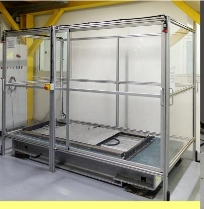
The Low Frequency High Stroke shaker is an innovative system based on liner motors system.
