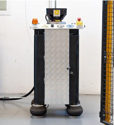
This machine allows the execution of mechanical semi-sinusoidal shock tests.
