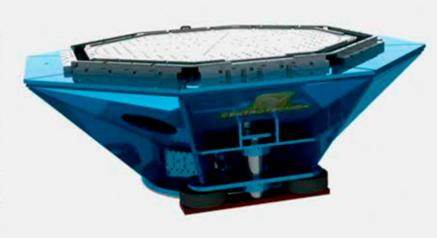
There is a perfect alignment between shaker armature motion and expander motion. The guidance is mounted and aligned on the machined frame, assuring precision and locking lateral and rotational expander modes. The guidance is completely mechanical, without oil or additional equipment, very low maintenance is therefore needed.
