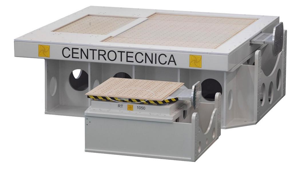
Our design department will consider any request to meet specific requirements for products not in the catalogue. In the example above: a large KRT slip table realized on specific request for combined climate + vibration battery testing, compared with a standard RT 1050 slip table.
