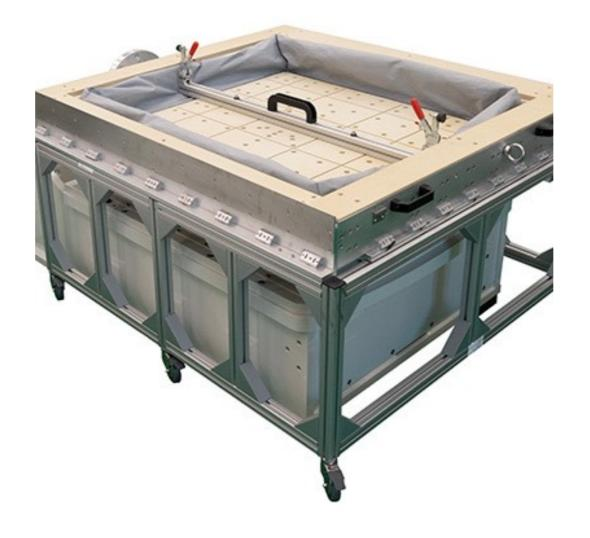
**Direct Coupling Solutions:** quick coupling system between climate chamber and slip table to take full advantage of the flexibility of slip tables (not just RTs).
