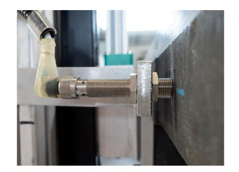
The **SENSORS SYSTEM** has been renewed with the use of a magnetostrictive position sensor.
