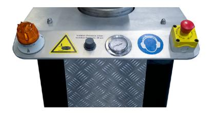
On the **CONTROL PANEL** of the machine there are the pressure regulator and the pressure gauge relating to the isolation of the machine from the ground.
