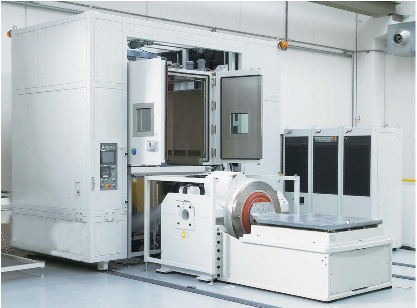
*Fig. 1: 74 kN Air Cooled Shaker
