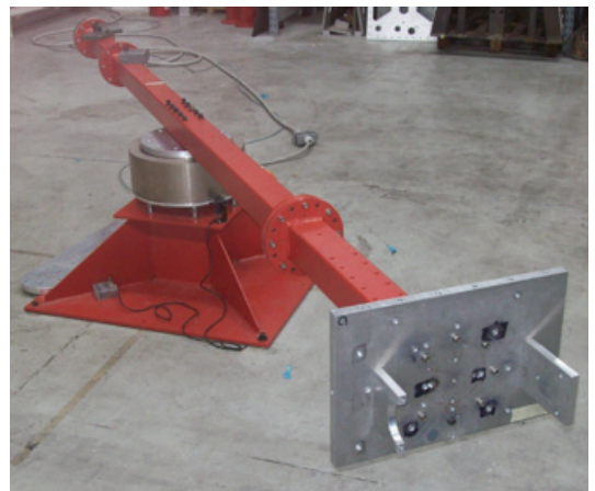
Fig. 2: Centrifuge System with interface plate
