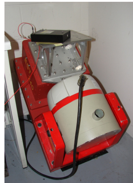
Fig. 3: V455 shaker with triaxial fixture for triaxial accelerometers calibration (+ item to calibrate)
